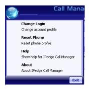
The Main menu screen menu item expands into an ability to Change the Login settings, an ability to reset the phone to its default settings, access help, and check the Call Manager version and serial number.
